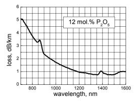
Fig.4. Optical loss spectrum in highly  $P_2O_5$ -doped single-mode fiber (cut off wavelength  $\lambda_c = 0.95 \ \mu$ m).
