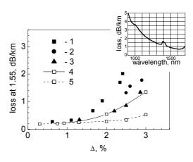
Fig.2. Fiber attenuation at 1550 nm for a series of  $GeO_2$ -SiO<sub>2</sub> core fibers. Closed symbols – [12]; open symbols – [3]. Insert: optical loss spectra in dip-free single-mode fiber doped with 26 mol.% GeO<sub>2</sub>.
