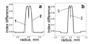
Fig.1. RIP of different types of  $GeO_2$ -doped fibers:1step RIP fiber; 2 – graded RIP fiber; 3 – graded RIP fiber with eliminated central dip.
