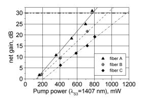
Fig.7. Variation of small signal net gain at 1500nm with input pump power: fiber A - HGDF; fiber B - NZ DSF; fiber C - LEAF.
