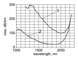
Fig.3. Optical loss spectra of single-mode germaniacore fibers: 1 - 97 mol.% GeO<sub>2</sub>, 2 - 75 mol.% GeO<sub>2</sub>.
