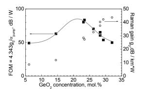
Fig.6. FOM and Raman gain dependence on GeO<sub>2</sub> concentration.
